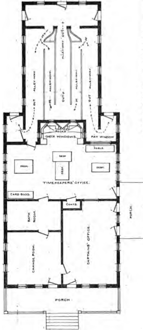
CAPTAINS & TIMEKEEPERS OFFICE SHOWING LAYOUT OF CHECKING WINDOWS, ALLEYWAYS ETC. NEWPORT MINE. NEWCASTLE, N.C.
